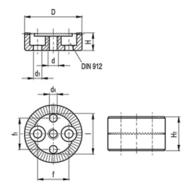
$$\begin{array}{lll} D & = 40 \\ d & = M8 \\ d1 & = 6.3 \\ d4 & H11 & = 6 \\ f & = 23 \\ f1 & = 23 \\ H & +/-0.9 & = 11.5 \\ H1 & = 23 \end{array}$$
